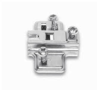
Zamak cruciform mounting plate with 30° inclination. Euro screws premounted. Vertical adjustment.
