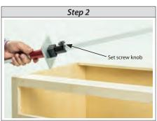
Make sure set screw knob is facing upward. Loosen set screw.
