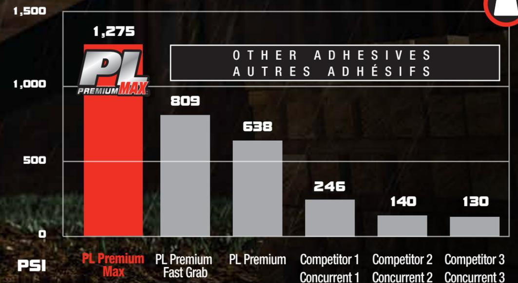
ASTM D3498 - Dry Lumber Adhesion / ASTM D3498 - Adhérence au bois sec
