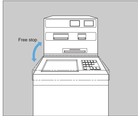
For opening/closing of maintenance machine doors.
