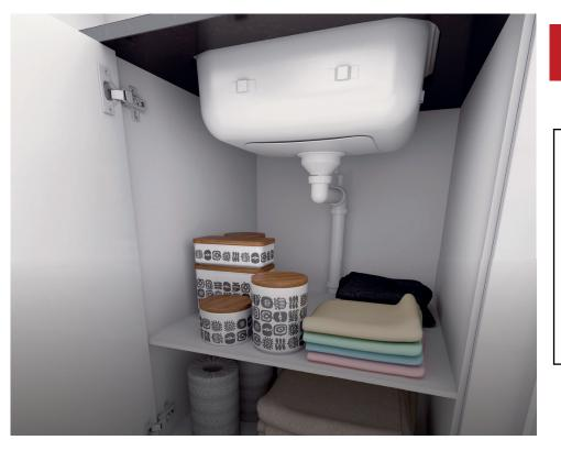
The Panama Siphon from RGX is a smart space-saving siphon. Panama is a complete drainage system which saves a lot of space in every cabinet. The P-Trap is replaced with an integrated recoil rubber valve, preventing gas and water from coming back up the drain.
