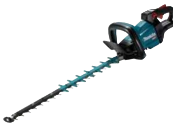
UH004GZ 40V max XGT 24" Hedge Trimmer Features sharp curved edge blade for trimming thin branches up to 15/16" 3-speed, reversible, electric brake, constant speed control
